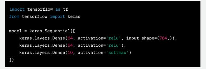
The above code defines a neural network with two hidden layers and an output layer. The **input\_shape** parameter of the first layer defines the shape of the input data.
